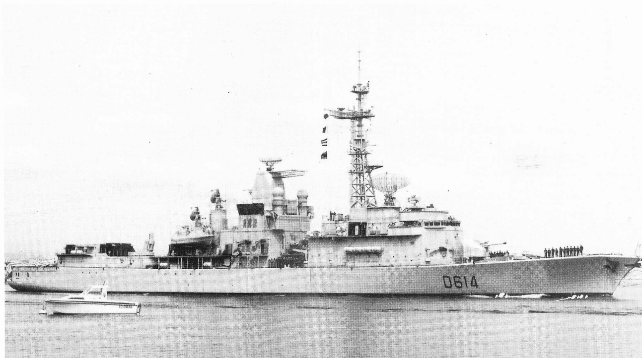
The French rocket destroyer CASSARD on a test run. The spherical housings forward of the funnel serve the satellite communication; the two devices arranged in order of their heights aft of the funnel are fire control components for the ship-to-air rocket weapons system.
